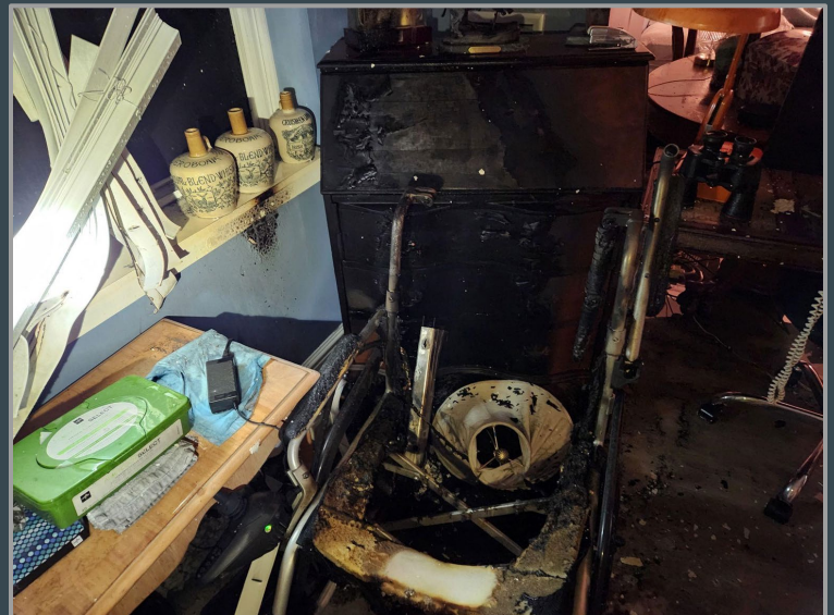
View of chair and the fire extension to the desk and curtains
