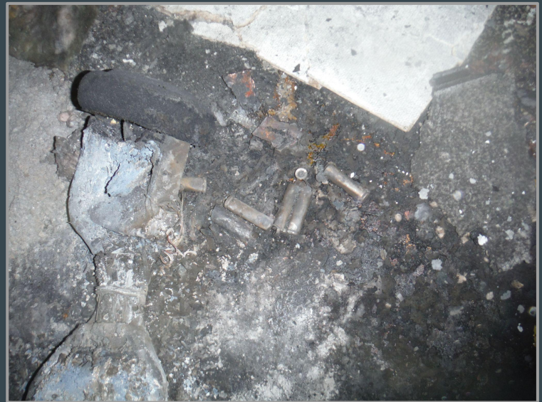
View of the hoverboard and catastrophic failure on the battery pack. Note the individual cells that were expelled from the battery pack
